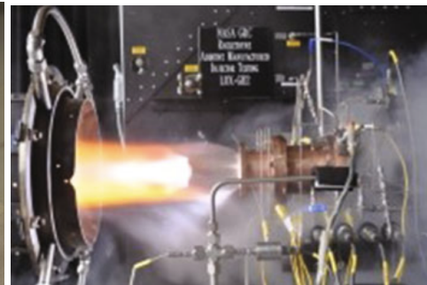
Figure 2.4: Testing of an Additive Manufacturing Rocket Nozzle
