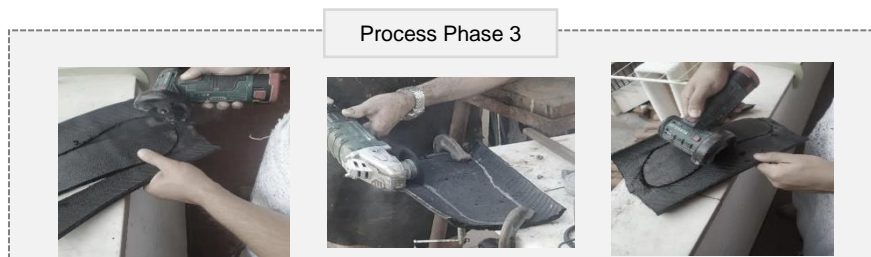
Figure 38 - Third process phase – Cutting soles from tyre
