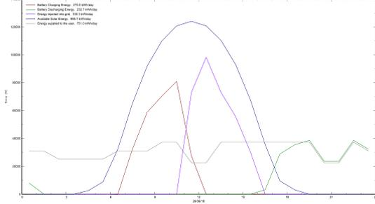
Figure 11: Hourly plot of the user’s needs (grey), PV system output (blue), grid-inject energy (purple), battery discharging energy (green), and battery charging energy (red), for a day in July.
