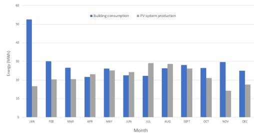
Figure 8: Monthly energy needs of the building and PV output energy, in MWh.
