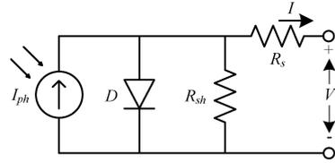
Figure 1: Equivalent circuit representing the one diode and five parameters model of the solar cell.
