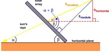
Figure 2: Components of solar irradiance on a tilted surface.
