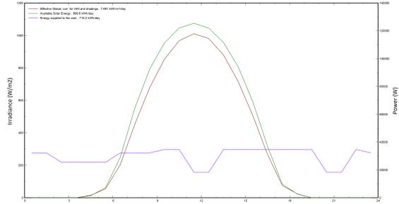
Figure 10: Hourly plot of the user’s needs (purple), effective global irradiance (red), and output of the PV system (green), for a day in July.
