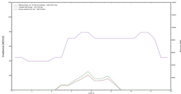
Figure 9: Hourly plot of the user’s needs (purple), effective global irradiance (red), and output of the PV system (green), for a day in January.
