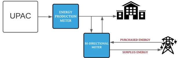
Figure 3: UPAC system connections and meter display.
