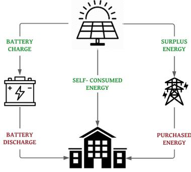
Figure 4: PV system interconnections and energy flows to grid, battery, and consumer.
