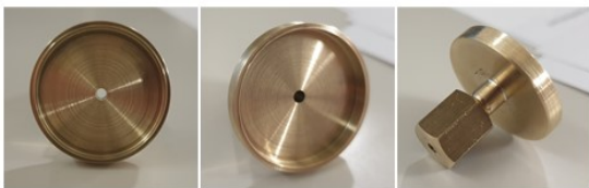
Figure 17: Feed cavity final constructed model
