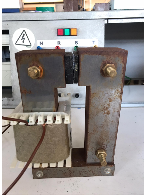
Figure 5.13: Experimental magnetic iron core circuit with YBCO
