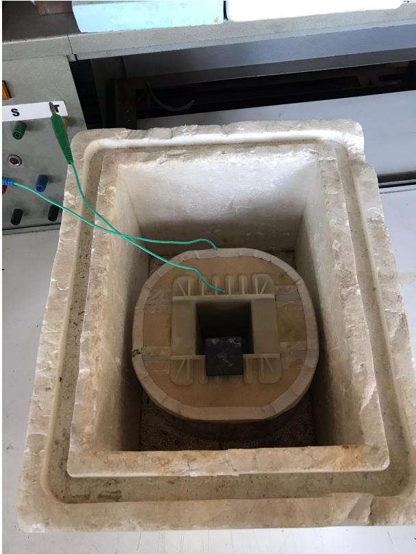
Figure 5.9: Experimental set up for coil with 4000 turns
