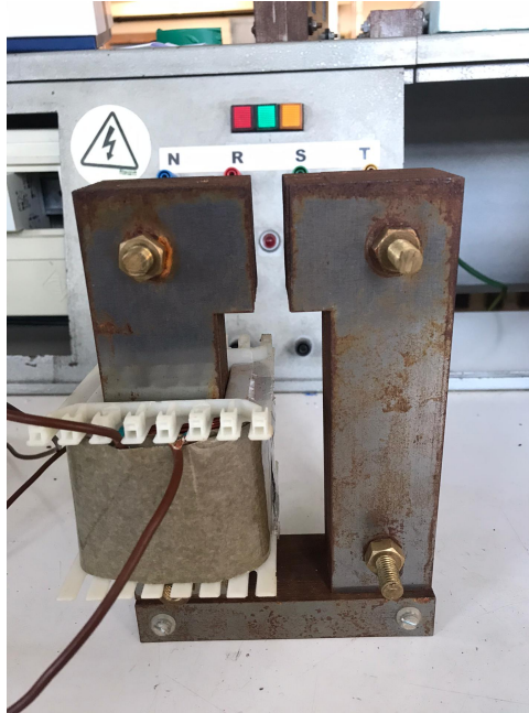
Figure 5.12: Experimental magnetic iron core circuit
