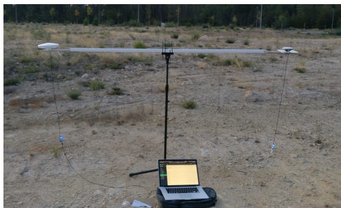
(a) Antenna configuration used in the static trials.
