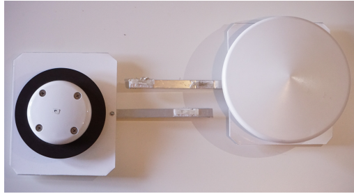
Figure 5.3: GPS antennas mounted with ground planes.
