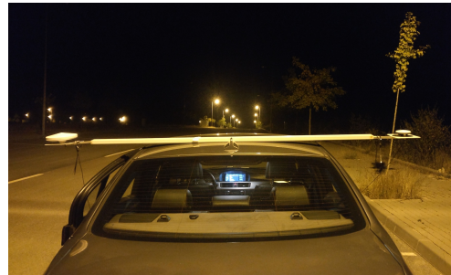
(b) Antenna configuration used in the dynamic trials.
