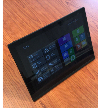
(b) Electronic Flight Bag (approx. 305 mm × 225 mm × 9 mm).
