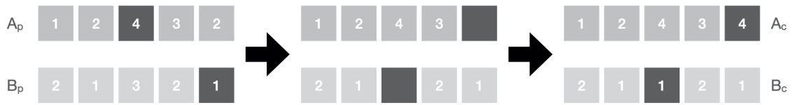
Figure 3.5: Example of the two-point crossover for machine assignment.
