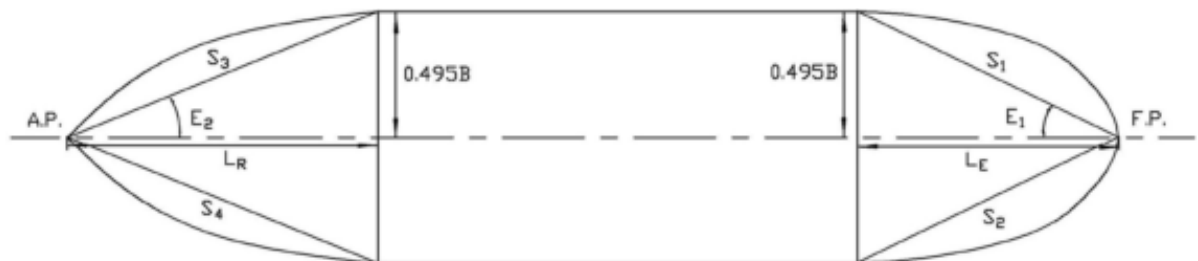
Figure 11 – Waterline and waterline parameters definition (Liu & Papanikolaou, 2020).
