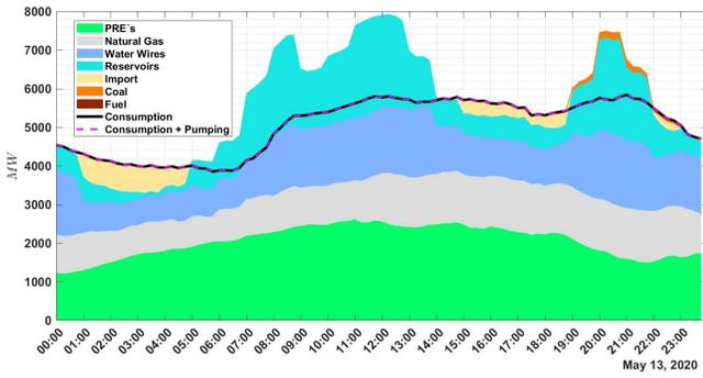
Fig. 5. Production and consumption diagram for May 13, 2020 (Source from [15]).
