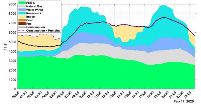
Fig. 4. Production and consumption diagram for February 17, 2020 (Source from [15]).
