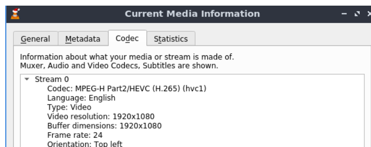
Figure 5.1: Video stream characteristics on the server side.
