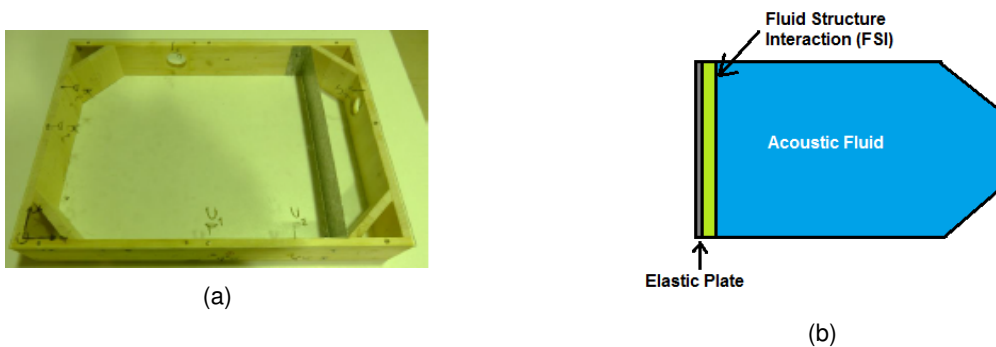
Figure 3.7: a) Experimental vibro-acoustic cavity [38]; b) Geometry of the numerical vibro-acoustic cavity.
