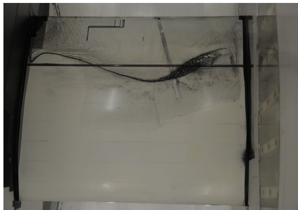
Figure 3.3: Oil flow for \alpha = 10^\circ
