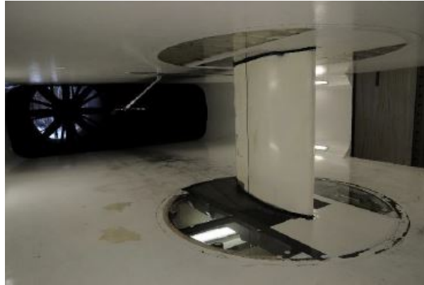
Figure 3.1: Wing Setup in the Laminar Wind Tunnel.
