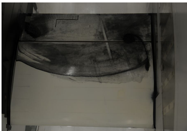
Figure 3.6: Oil flow for \alpha = 16^\circ
