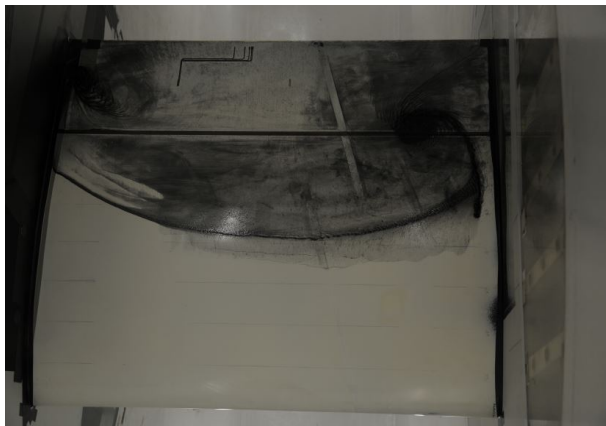
Figure 3.5: Oil flow for \alpha = 15^\circ
