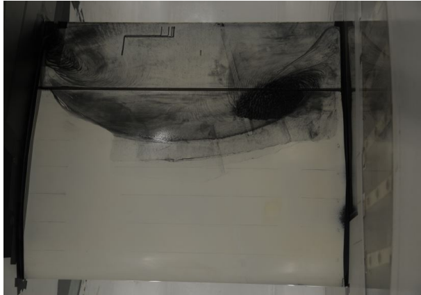
Figure 3.4: Oil flow for \alpha = 12^\circ
