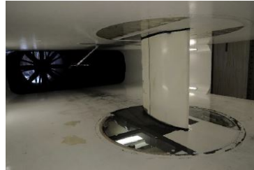
Figure 2: Wing Setup in the Laminar Wind Tunnel.
