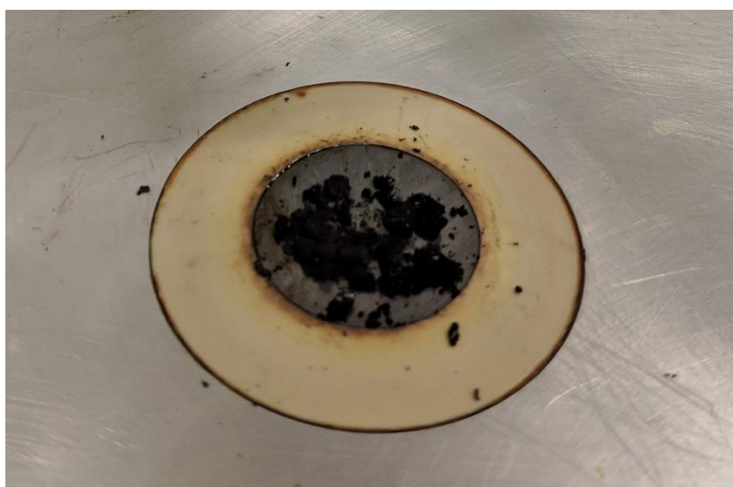
Figure 38: Sample of a residue treated with alkylphenolic removal treatment
