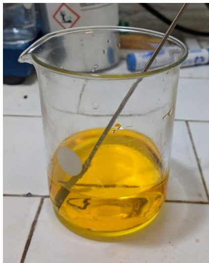
Figure 35: Mixture of 5% DMAP in acetic anhydride
