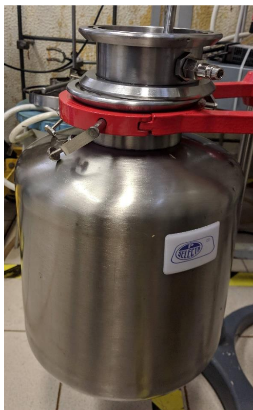
Figure 33: Reactor Selecta 6 L. Coil was put on the top of the reactor
