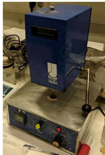
Figure 29: Viscometer REL CPD 2000
