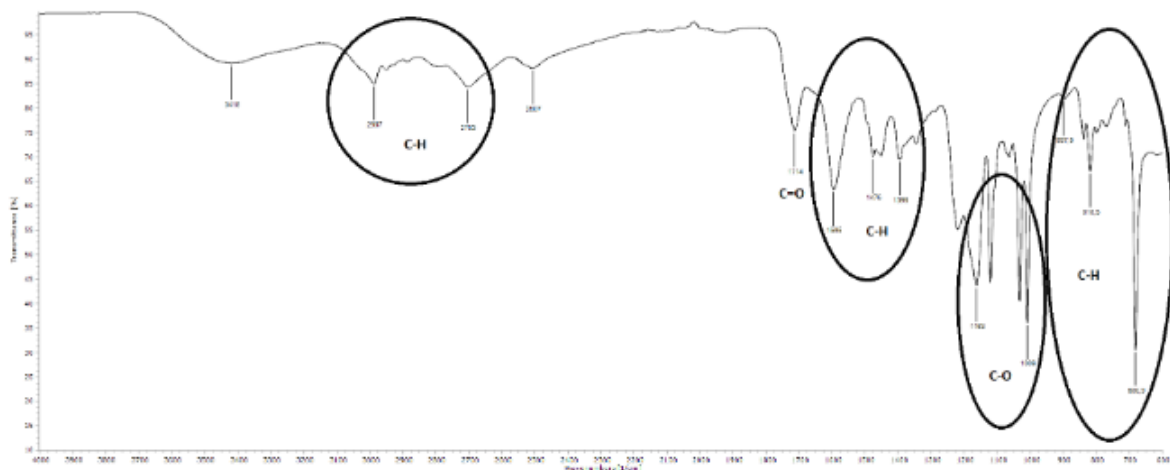
Figure 39: Perkin-Elmer screenshot of liquid sample filtrated after TEA treatment
