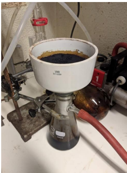
Figure 30: Filtration apparatus connected to vacuum pump
