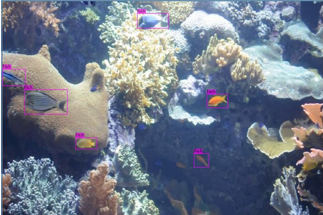
Figure 2.3: Output for the frame in 2.1 after running it through the object detector YoloV3 [27], with the bounding boxes shown in pink.
