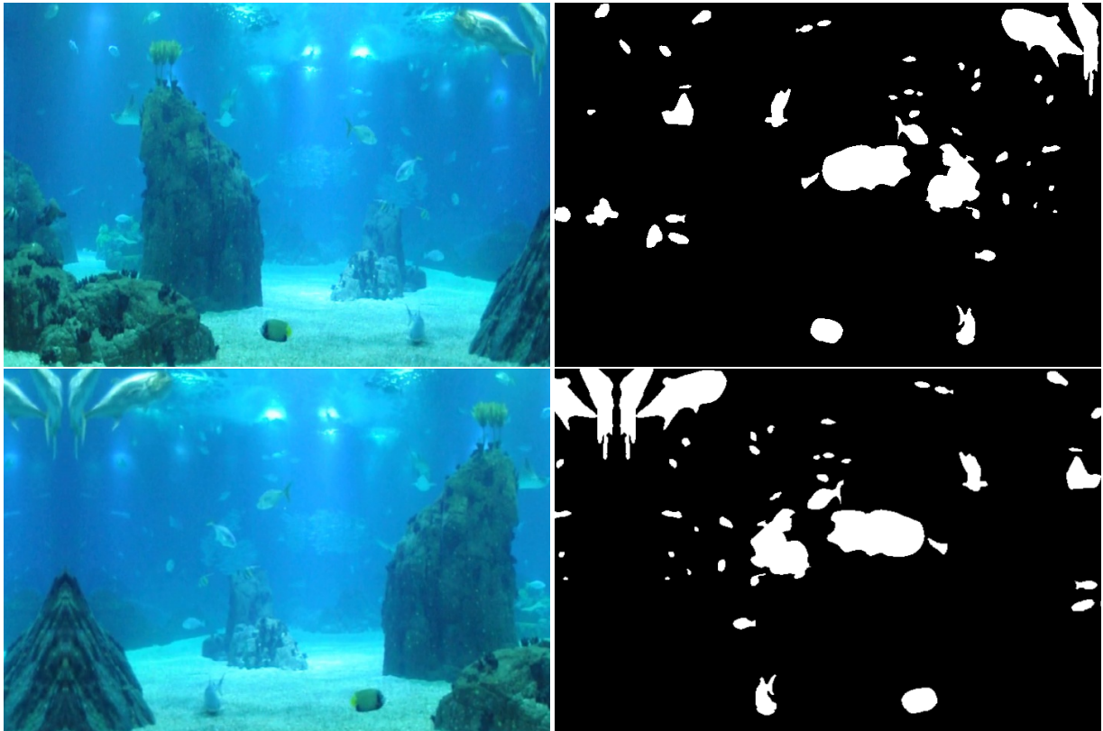
Figure 5.1: Top row: Original frame and corresponding segmentation; Bottom row: Frame and segmentation after augmentation using width shifting, horizontal flipping and zoom.
