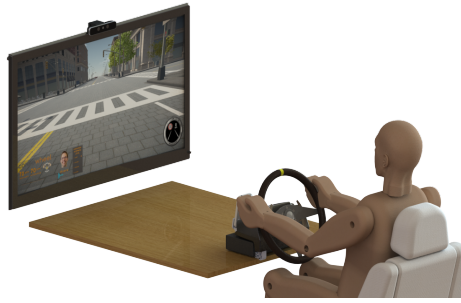
Figure 1.2: Driving simulator setup: A computer simulated environment is presented in the screen, while the driver controls a vehicle using the pedals and CardioWheel. The simulator not only integrates the inputs to run the environment, but also aggregates inputs from the wheel movements, CardioWheel sensor, and intel realsense camera to a database.
