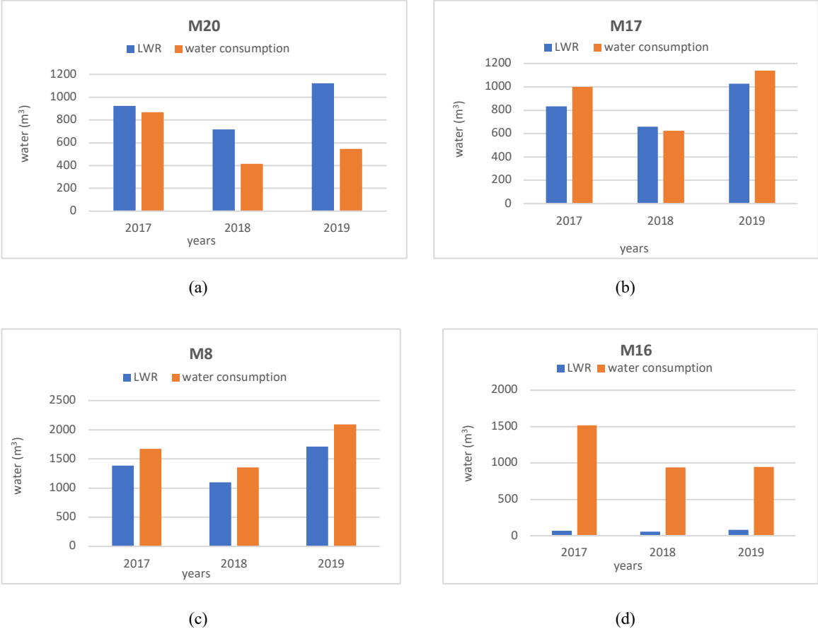
Figure 5-12 Vale do Lobo irrigation efficiency in 2017, 2018 and 2019: LWR versus water consumption for the irrigation meters (a) M20, (b) M17 (c) M8 and (d) M16.
