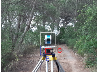
Fig. 3: Low Cost stationary LiDAR system. This system is composed by the LiDAR sensor (A), a turntable (B) and a step motor (C).
