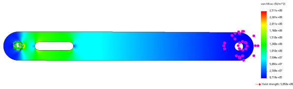
Figure 8: Stress plot of the Petal in the AUV mechanism (deformation scale of 7).
