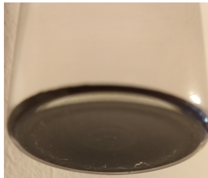
Figure 4.26: Precipitate of silver oxide in the silver nanofluids.
