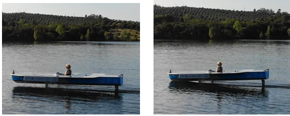
(a) Flight just after takeoff and (b) Moment where the boat "bow dives".
