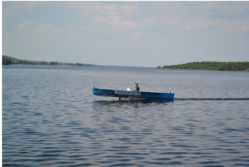
Figure 7.8: Flying with small rear AoA.
