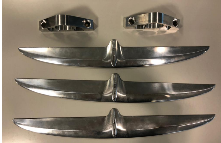
Figure 2.2: The hydrofoils designed for SR01 that will be used on SR02.
