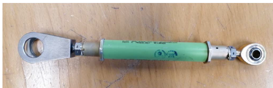
Figure 8: Tie rod sample tested until tensile failure.
