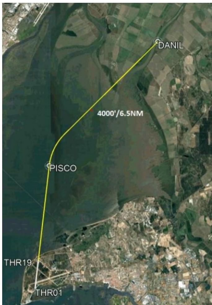
Figure 6.2: Departure proposal for track 01 with 10% climb gradient [7]
