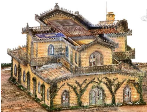
Figure 5 – Final ordered point cloud of the Chalet of the Countess of Edla
