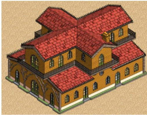
Figure 7 - H-BIM final model of the Chalet of the Countess of Edla, in software Autodesk Revit
