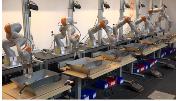
Figure 2.3: QT-Opt: Seven identical robots autonomously collect grasping episodes [17]
