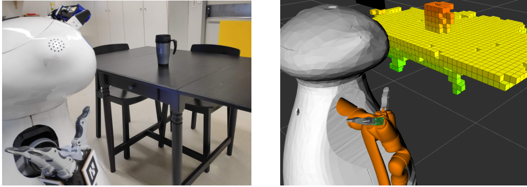
Figure 4.5: Octomap representing the environment's occupancy volume.
