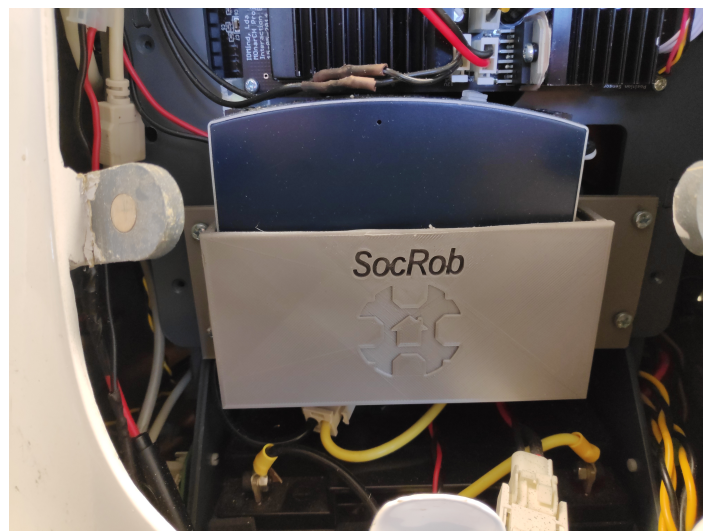
Figure A.8: Converter inside MBot, held by the 3D-printed pocket.
