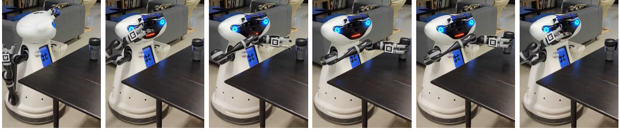
Figure 5.5: Steps of a grasping episode. Left to right: sweeping head, pregrasping, visual servo start, visual servo end and closing fingers, lifting object, moving back to resting pose after lowering object and opening fingers
