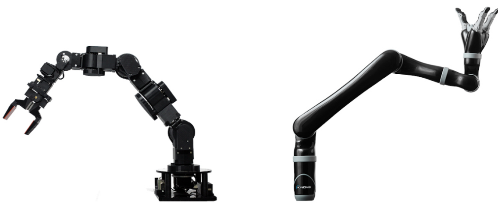
Figure 4.1: Left: Cyton Gamma 1500, previously used in MBot. Right: Kinova Gen2, the arm used in our work.
