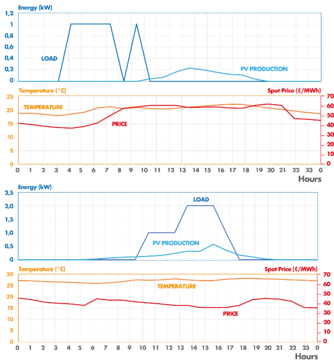
Figure 7 - Energy load (blue line), PV production (light blue line), Temperature of the room (orange line) and Spot Price (red line) using smart MPC during 2 summer days in Lisbon
