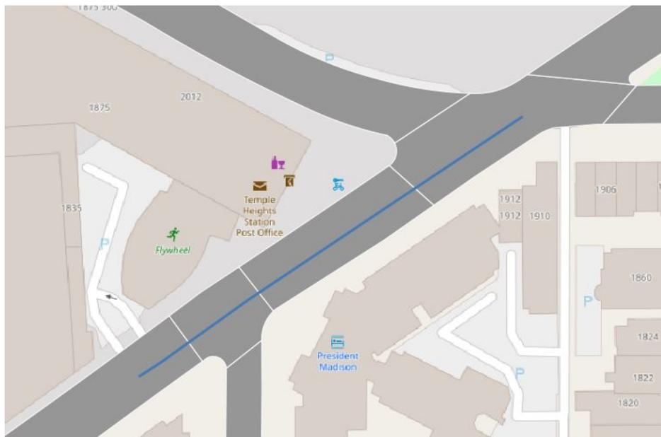
Figure 3.1: The visual representation of a group of road polygons (grey) intersecting with a specific road segment linestring (blue)
