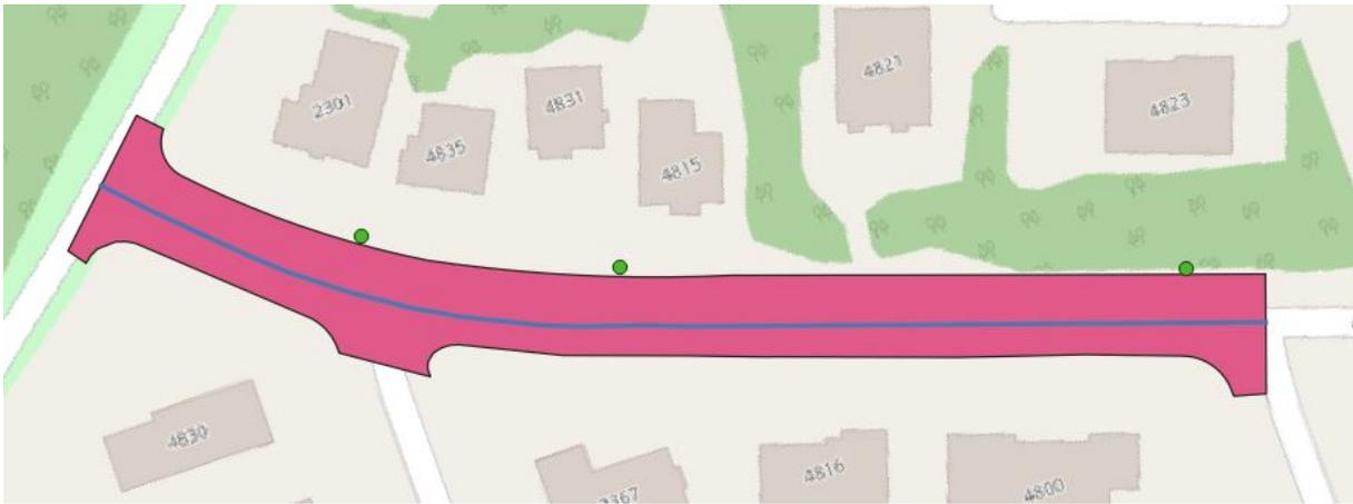
Figure 4.23: Example of a road segment with spacing uniformity disrupted by an absence of a street light in a sequence
