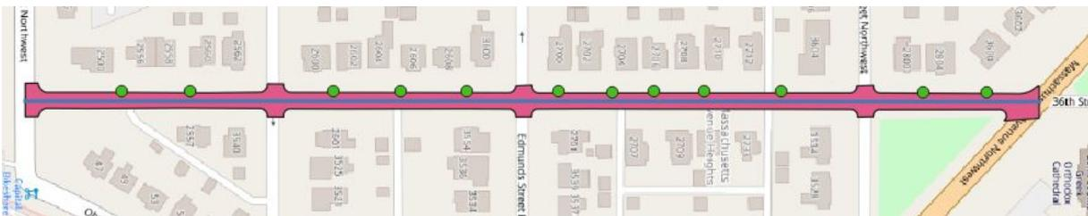
Figure 4.24: Example of a road segment with spacing uniformity disrupted by intersections
