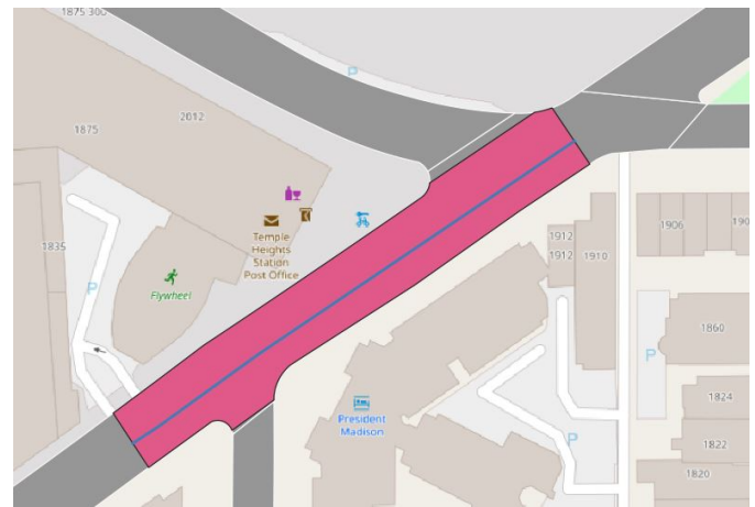
Fig. 1. The union of polygons (violet) intersecting with a specific segment's linestring buffer (blue)
