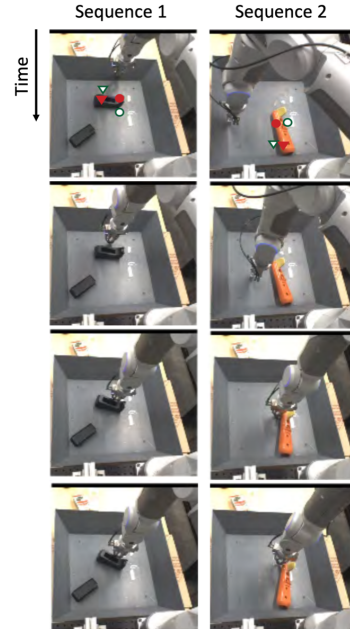
Figure 3.3: A robotic arm using Visual MPC to push objects from an initial position (in green) to a designated goal position (in red). Source [60].
