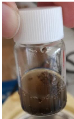
Figure 24 – Solubility test of the biomass in water.
