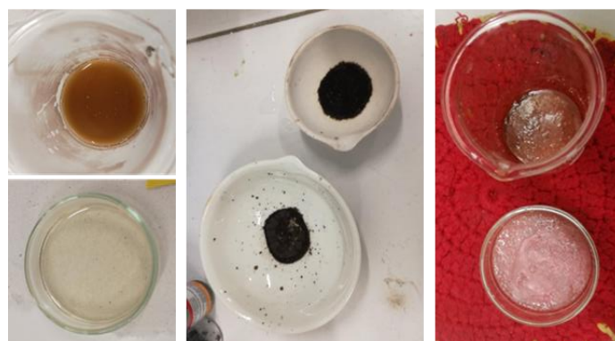
Figure 47 – FP6 (down) and FP7 (top) before (left), after drying at 300 °C (middle) and after drying at 50 °C (right).
