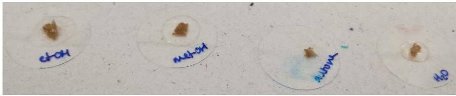
Figure 37 – Solubility test to Q1 with ethanol, methanol, acetone and distilled water (left to right).
