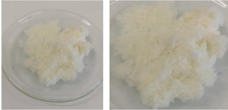
Figure 45 – FP4 before (left) and after (right) drying in a 50 °C stove overnight.
