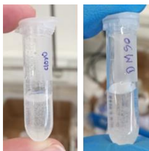
Figure 36 – Solubility test to chitosan commercial with chloroform (left) and DMSO (right).
