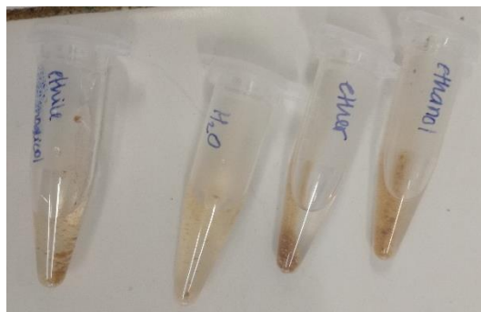
Figure 40 – Solubility test to Q3 with ethylene glycol, distilled water, ether and ethanol (left to right).
