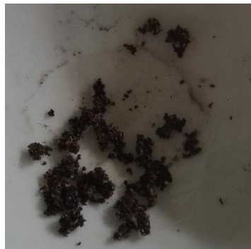
Figure 46 – FP5 after drying 2 hours in a 130 °C muffle.
