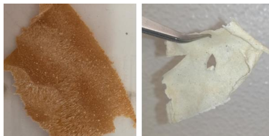
Figure 68 – PG33 before (left) and after (right) left under direct sunlight.
