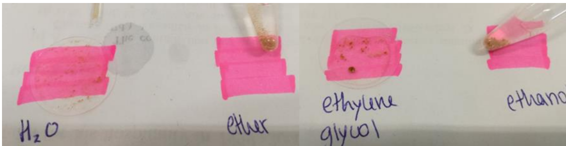
Figure 39 – Solubility test to brown Q2 with distilled water, ether, ethylene glycol and ethanol (left to right).
