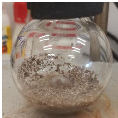
Figure 16 – Chitin stirred with a solution of NaOH 60 %.
