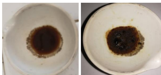
Figure 50 – FP12 after the first (left) and second (right) time drying at 130 °C for 1h30 in the muffle.
