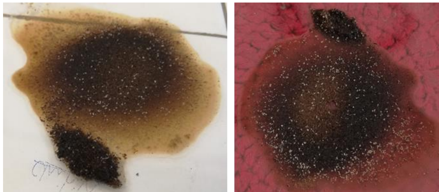
Figure 44 – FP3 after drying in a 50 °C (left) stove and in a 130 °C (right) muffle.
