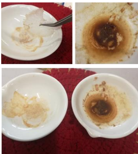
Figure 48 – FP8 (left) and FP9 (right) after drying at 130 °C in the muffle the first (top) and second (bottom) time.
