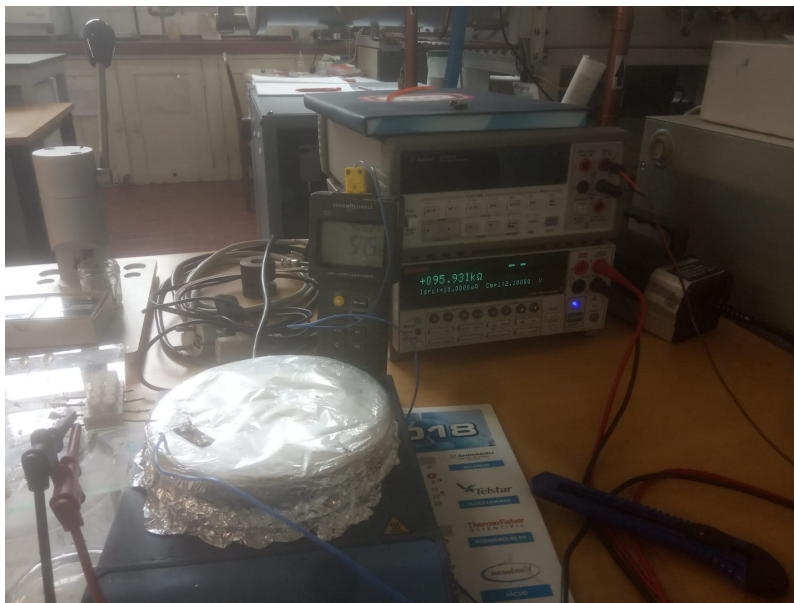
Figure 32: Picture of the setup for electrical resistance measurement with temperature variation.
