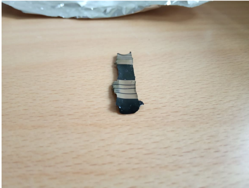
Figure 30: PDMS/carbon nanotube sample with two sets of deposited gold electrodes. Typical dimensions (width: 6 mm, thickness:1 mm, length: 2 cm).
