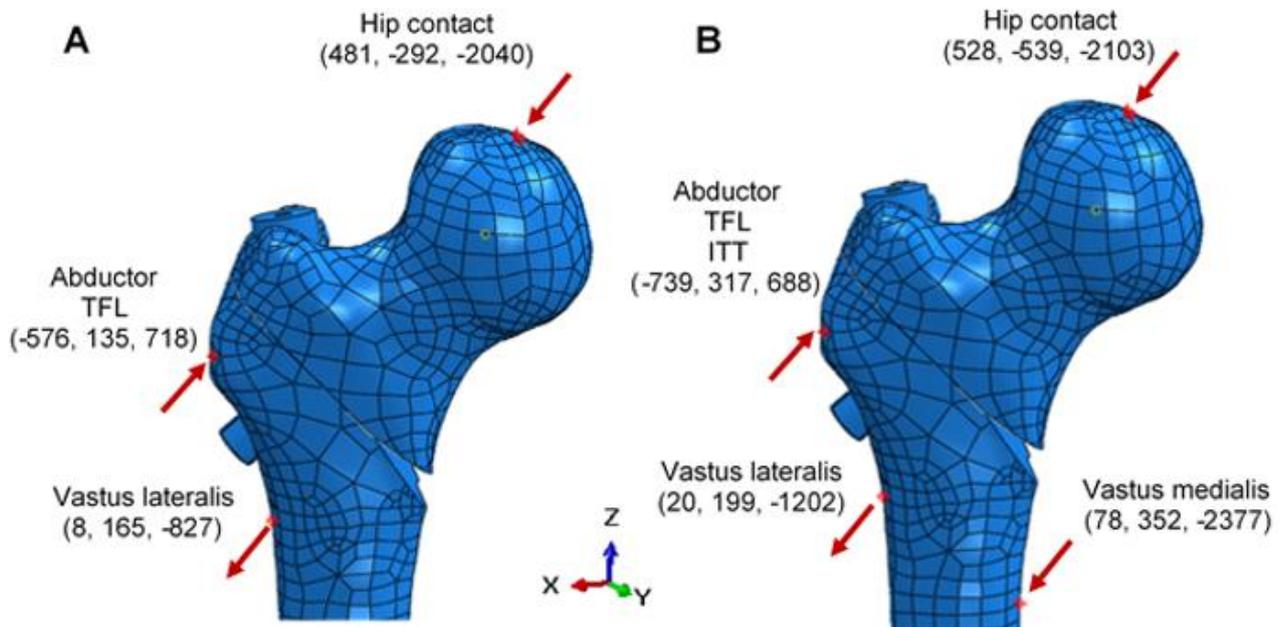
**Figure 2** – Identification of the application points and the loads' magnitude: (A) normal walking case (B) stair climbing case.
