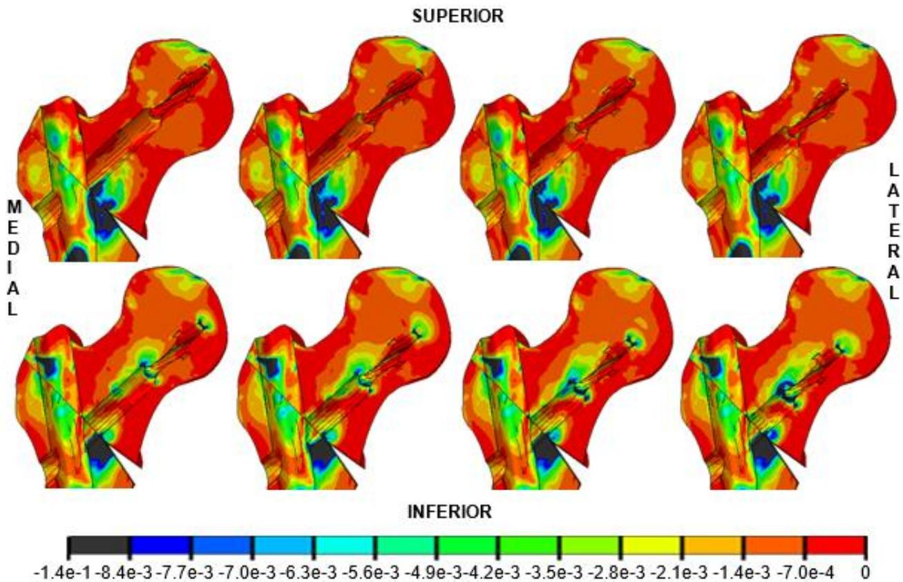
**Figure 3** - Minimum principal strains in a coronal section of the proximal region of the femur for the stair climbing case. The minimum of the strain scale is defined as the yield strain of the human bone (-0.84%) to emphasize the regions of the bone more susceptible to undergo irreversible deformations (black areas).
