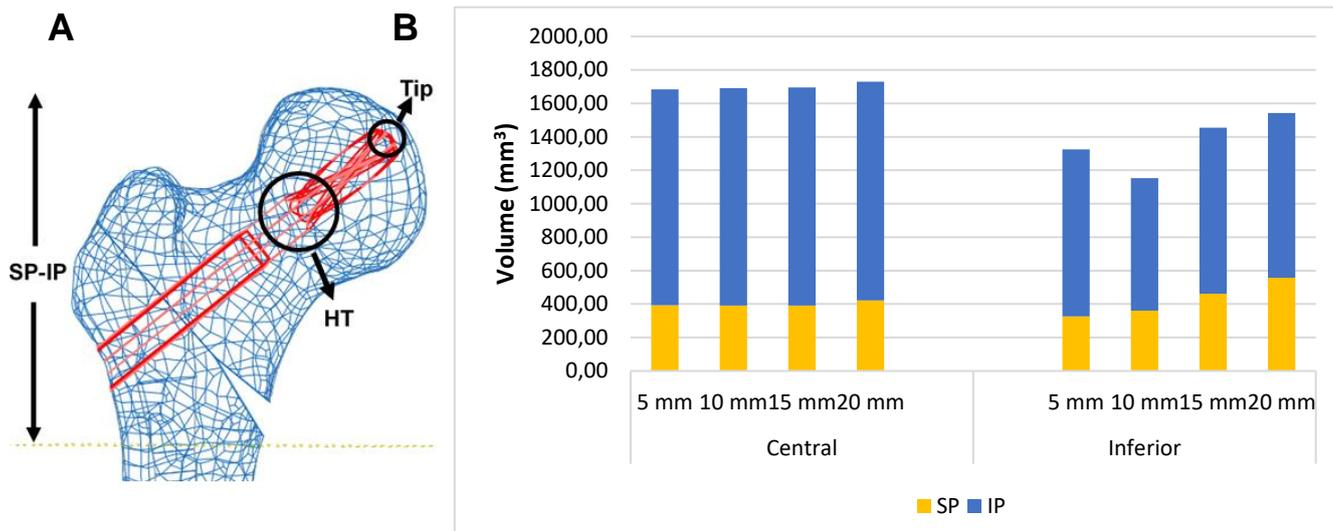
**Figure 4 –** (A) Representation of the SP-IP Region (bone above the dashed green line), Tip Region (bone inside the sphere at the tip of the blade) and HT Region (bone inside the sphere around the head-tail transition). (B) Volume of bone in the SP-IP Region with minimum principal strains below the compressive yield strain of 0.84%. The contributions of the superior (SP) and inferior (IP) parts are also detailed.
