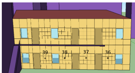
Figure 5.6 – Division of the façade of Building 2 into smaller surfaces.
