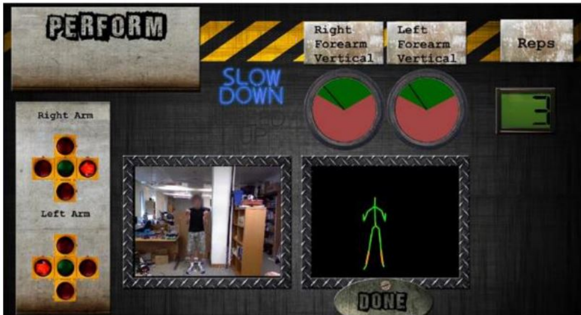
Figure 2.2: MotionMA - Performance interface. Information regarding static bones is displayed on traffic lights whilst the ranges of motion of dynamic bones are displayed on dials. The user can see the video recording of the demonstration and his own skeleton as tracked by the Kinect with each bone in a different colour depending on its score. The interface also displays the repetition count and warnings when the speed is too fast or too slow [5]
