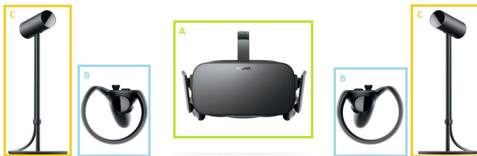
Figure 4.2: Oculus Rift Hardware: A - HMD; B - Touch Controllers; C - Position Trackers.
