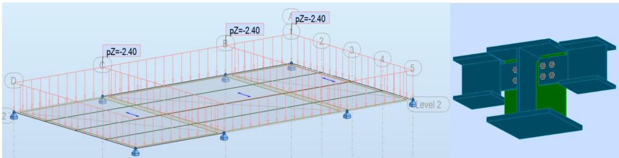
Figure 7: Composite Slab model in Robot Structural Analysis and steel connection between beams.
