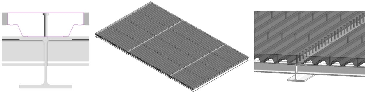
Figure 8: Modeling of the profiled steel sheeting, concrete layer and shear connectors.
