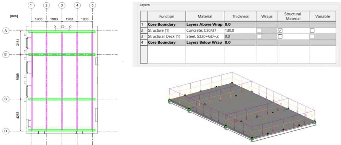
Figure 5: Composite slab parametrization.
