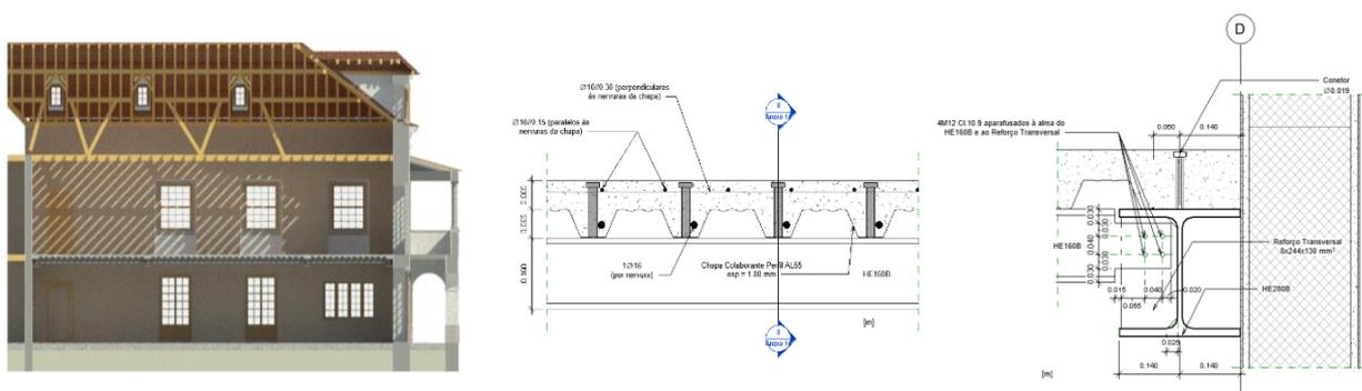
Figure 9: Cut and schematic drawings of the composite slab.
