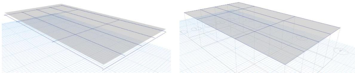
Figure 6: Composite slab transposition to *ETABS*: 1<sup>st</sup> Attempt and 2<sup>nd</sup> Attempt.
