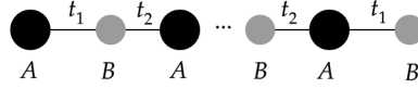
Figure 3.2: SSH chain. Each unit cell is composed by two distinct sites, A and B . t_1 is the intracell hopping amplitude, and t_2 is the intercell hopping amplitude. t_1 and t_2 might be complex.
