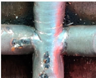
Figure 13: Necking effect found on areas adjacent to the intersection area.
