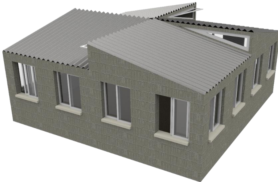
F37 – Cross Ventilation Scheme with added roof windows in a 0.3 glazing ratio house (south-eastern perspective view).
