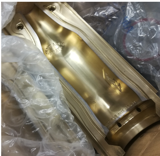
Figure 2: Example of engravings and light diffuse reflection in a bronze mold - Ref. 2283 female
