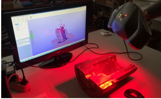
Figure 9: Cast iron mold being scanned with ZS-scanner 700 with position targets at Lab2ProD
