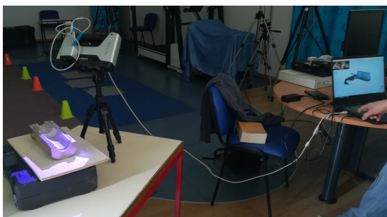
Figure 10: Einscan-Pro in fixed mode
