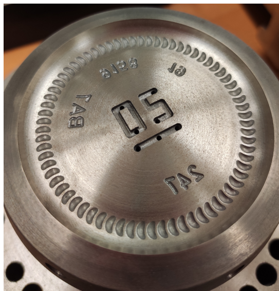
Figure 2.5: Example of engravings that can be present in bottle molds - Bottom part of Ref.9158
