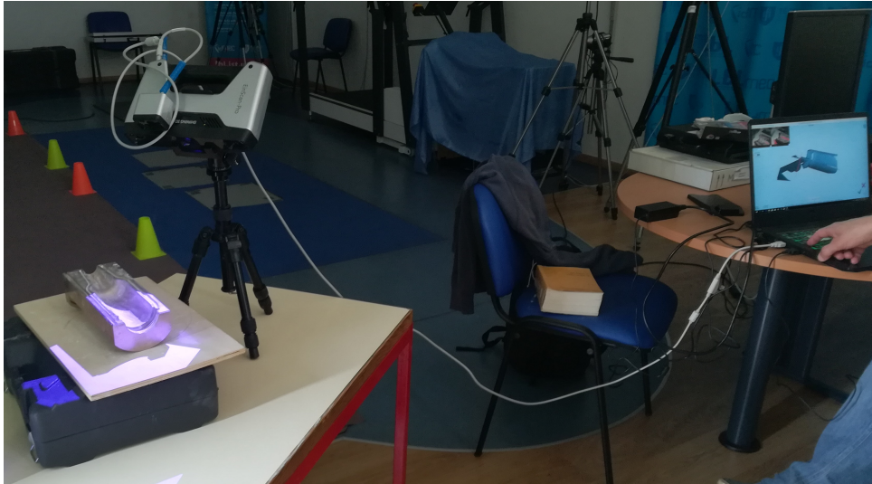
Figure 4.6: Einscan-Pro in fixed mode
