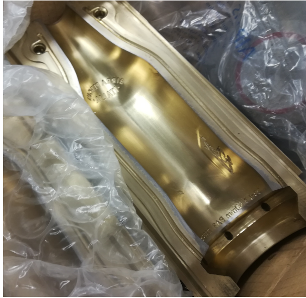
Figure 2.7: Example of engravings and light diffuse reflection in a bronze mold - Ref. 2283 female
