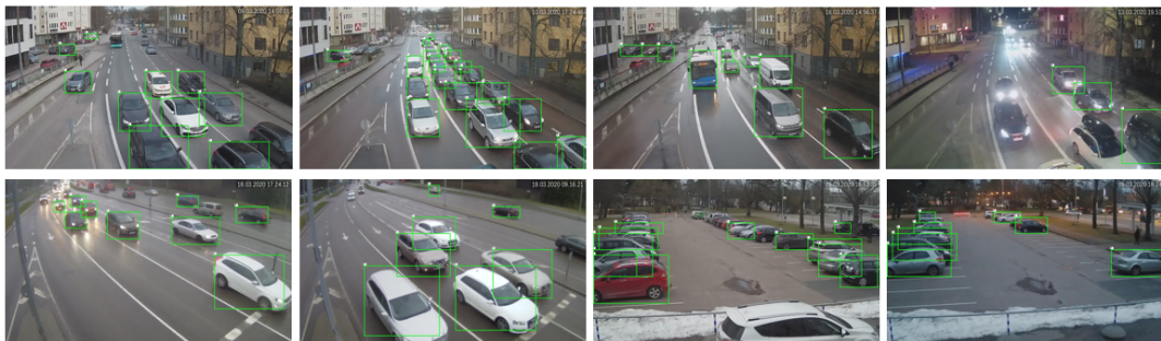
Figure 6. Detections made by our model on the Tallinn traffic dataset.
