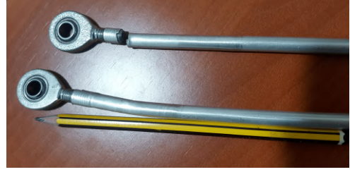
Figure 2: Damage occurred during the assembly of the first sensing bars.
