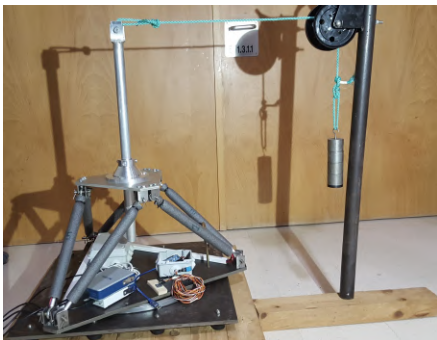
Figure 12: Apparatus with a pulley to create a F_X .
