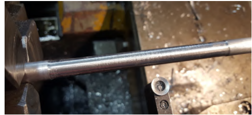
Figure 3: Manufacture of the new sensing bar
