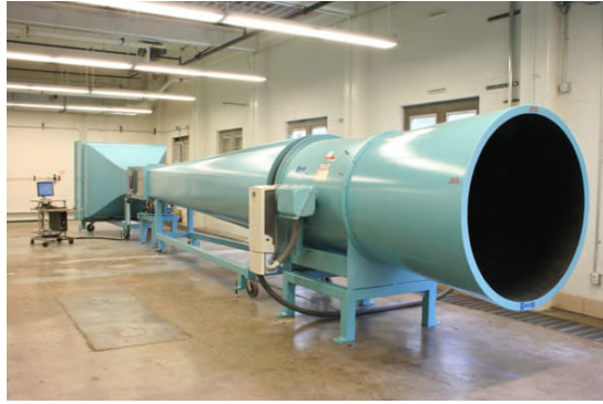
Figure 1.5: Example of a wind tunnel. Courtesy of Aerolab.
