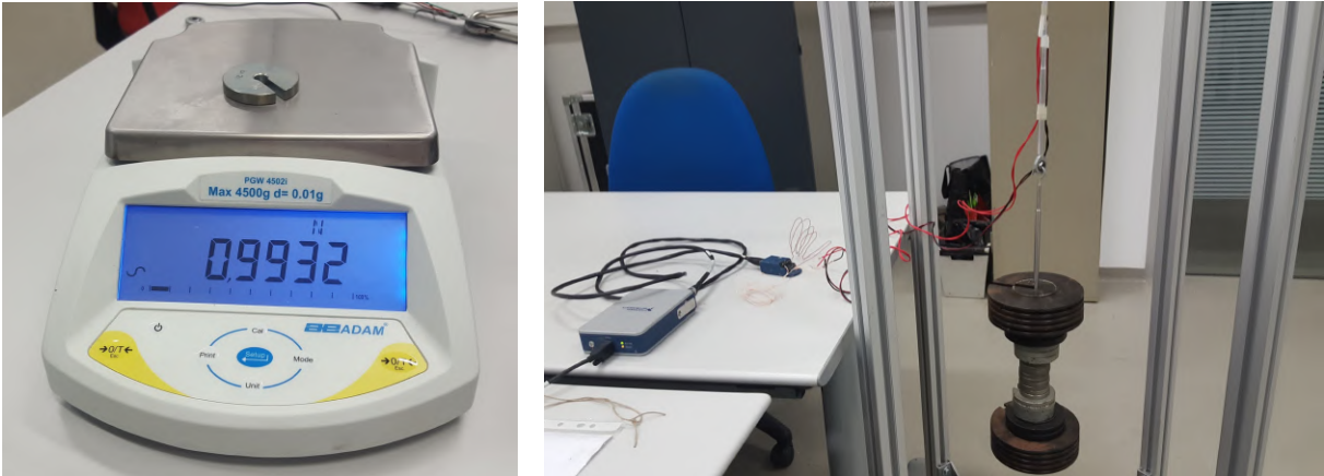
(a) Weighing of an increment weight to setup the load set. (b) Experimental apparatus with support, complete load set applied and NI 9237 board as DAQ.
