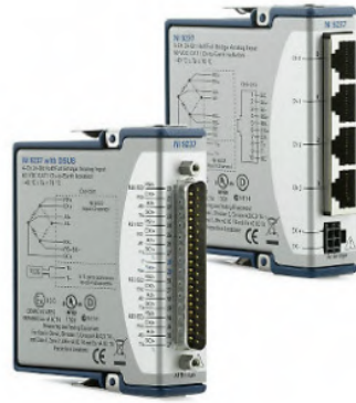
(a) NI 9237, which DSUB and RJ45 gates, by National Instruments™ [27].
