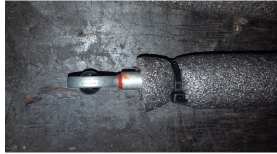
(b) Fixation of sensing bar and rod end bearing using glue.
