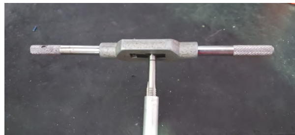
(b) Creation of female thread with a tap tool.
