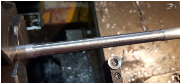
(a) Machining with a lathe and a circular turning insert.
