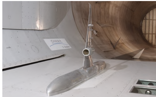
(b) Aircraft half model. Courtesy of ONERA.
