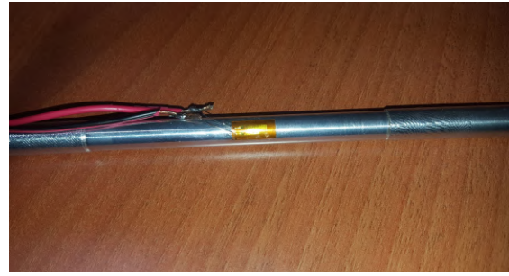
(b) New sensing bar made only for experimental tests.
