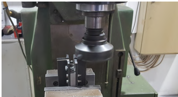
(a) Milling of the pitot support fixation.
