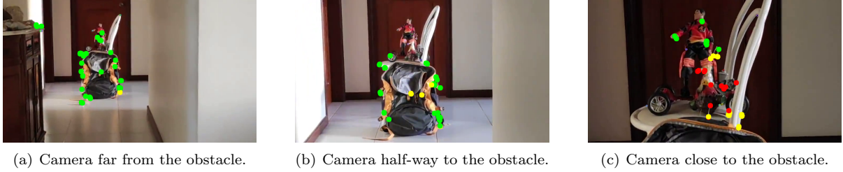
Figure 9: Three different stages in a hall 'flight'. The colored dots correspond to the marked matches by the vision algorithm with the following TTC: Green points: TTC > 8s . Yellow points: 4s < TTC \leq 8s . Red points: TTC \leq 4s .
