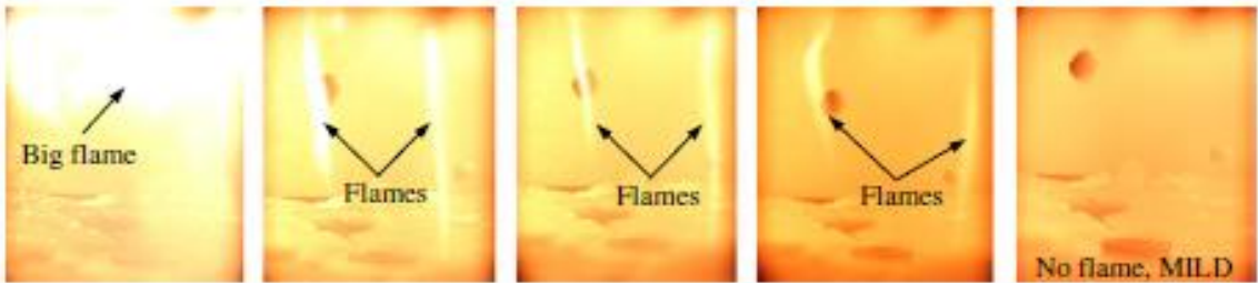
Figure 2.2 - Transition from conventional combustion regime to flameless combustion regime (adapted from [14])
