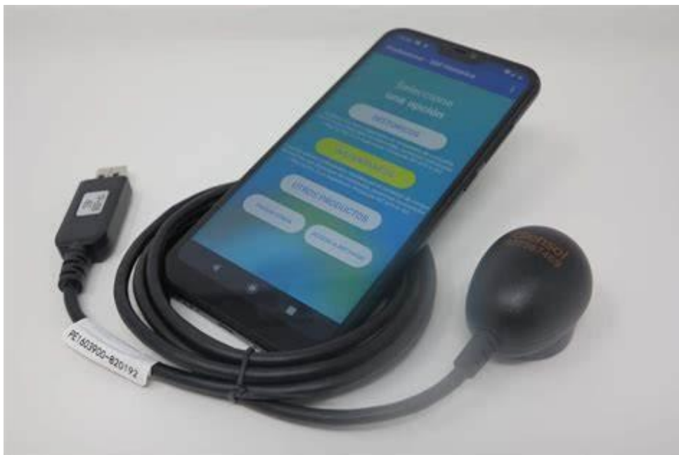
Figure 3.3: Kit IEC to download data from electric meter to mobile.
