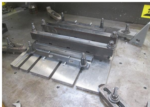
Figure 3.5: Clamping system fastened.
