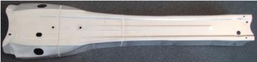
Figure 2.12: Centre tunnel of the Mercedes-Benz SL R231, from [35].
