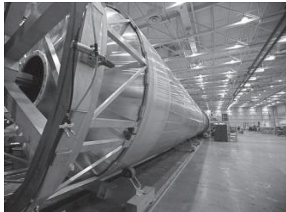
Figure 2.11: Falcon's 9 tank manufacture with circumferential and longitudinal friction stir welds, from [33].
